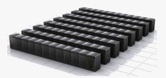
Multi-rack system Mira: 48 racks, 10 PF/s Geometry: 8x12x16x16x2
