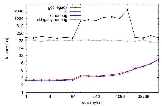
OSU MPI Multi-threaded Latency Test v3.6 (internode)
