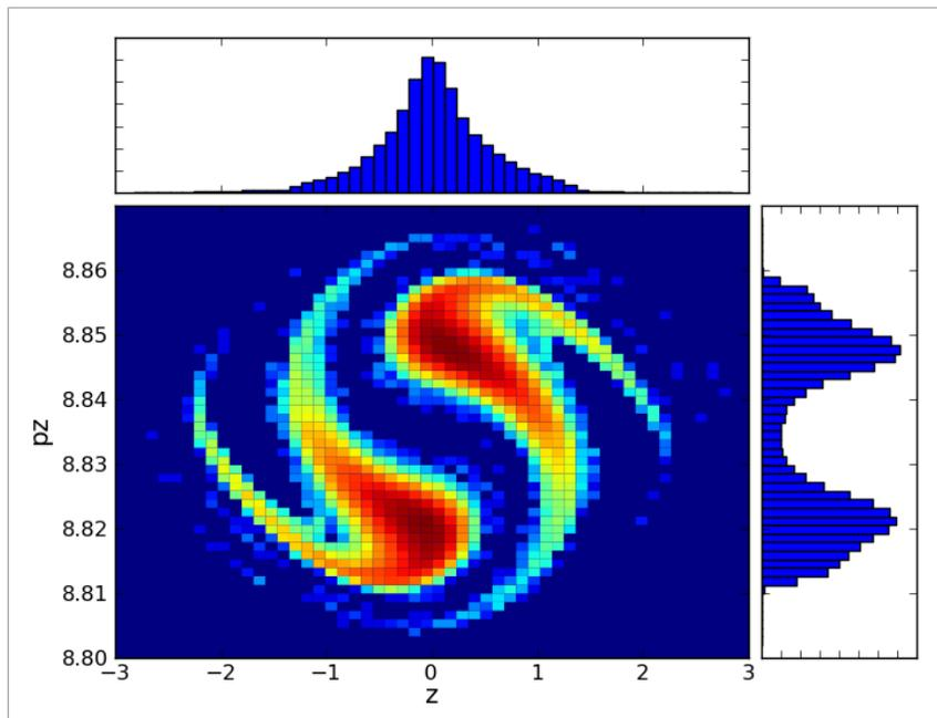
**Figure 3.1** Slip-stacking simulation in the Fermilab Recycler. Two injected batches of bunches are combined to form a batch of high-intensity super bunches.
