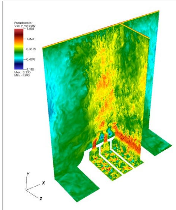
Figure C.5 Vertical velocity calculated by Nek5000 in the triple-jet thermal mixing experimental benchmark WAJECO.
