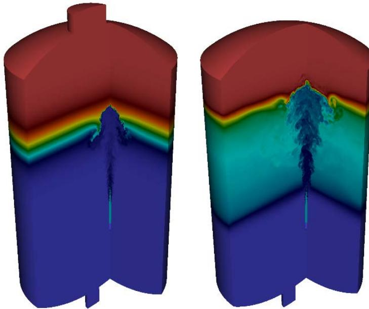
Figure C.6 This visualization depicts the helium mass fraction (red=high, dark blue=low) of the mixture inside the PANDA containment at early time (*left*) and late time (*right*). At late times, the helium has mixed with the lower air-rich layer significantly and has also completely penetrated the air-helium stratification layer.
