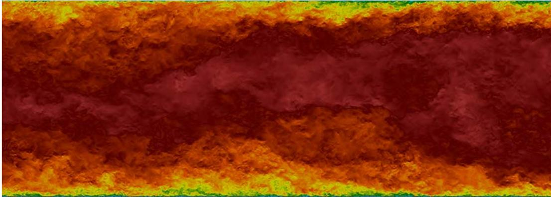
Figure 3.5 A visualization of the instantaneous streamwise velocity component over a section of the simulated channel.
