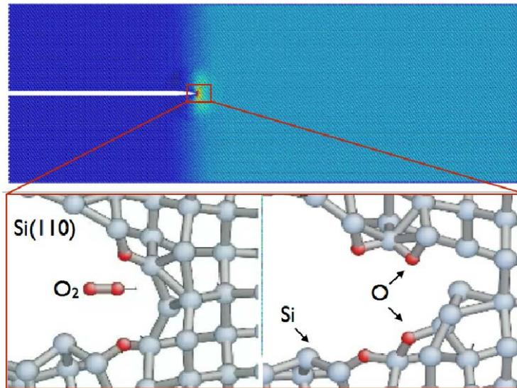
Figure 3.4 (Top) Stress corrosion cracking in the Si (110) cleavage system. Model system, colored by principal stress, with red regions corresponding to high tensile stress and dark blue regions to zero; the red rectangle represents the region shown in the bottom panel. (Bottom) Crack tip structures obtained by QM-MM geometry optimization.
