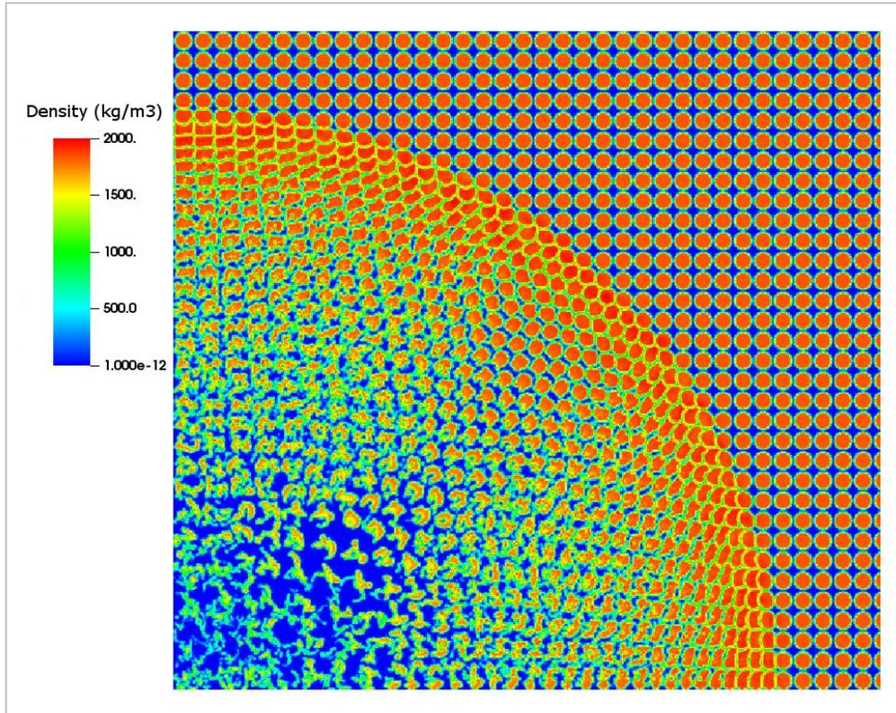
Figure C.1 Proposed DDT mechanism of inertial confinement. This image shows the density of the explosive cylinders late into the simulation.
