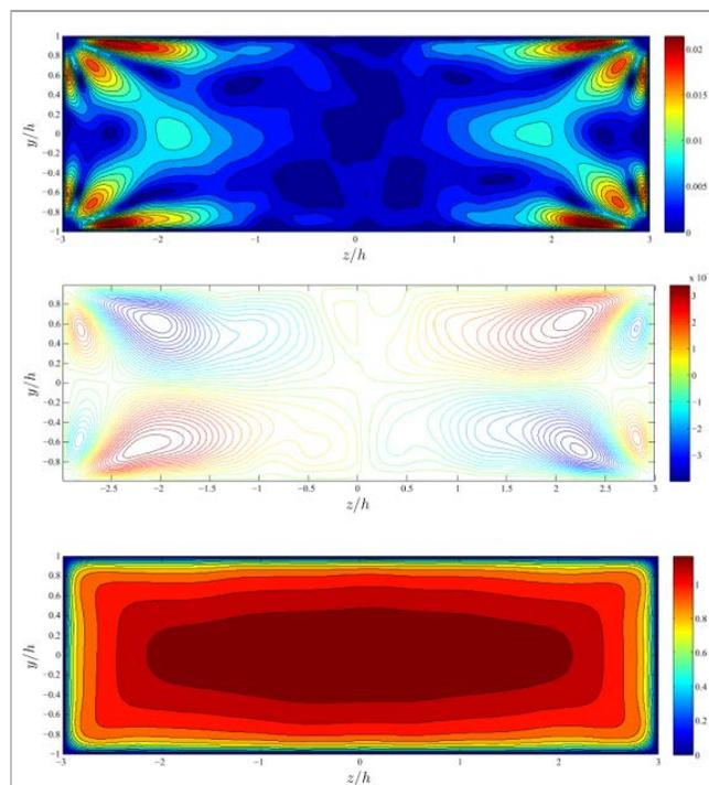
Figure C.10 In-plane velocity, streamlines, and streamwise velocity of the aspect ratio 3 case.
