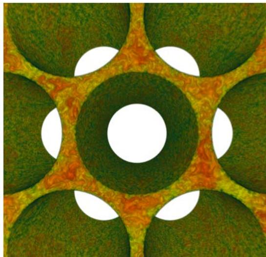
**Figure C.4** Nek5000 velocity results for 37-pin rod bundle of Krauss and Meyer experiment. Results depict the range of scales (and hence the large number of degrees of freedom) needed to resolve small features and accurately calculate wall-shear stress in large eddy simulations.
