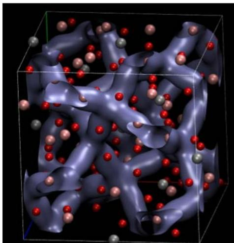
**Figure C.3** An image of the LLZO material (200 atoms). The tubes depict iso-surface representations of the free-energy surface of Li-ion conductivity. Within the tubes, Li atoms (pink) can be observed moving inside the material.
