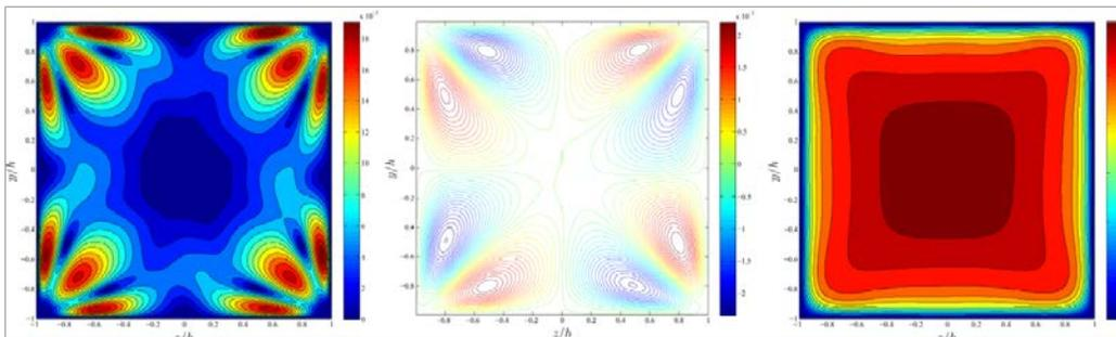
Figure C.9 In-plane velocity, streamlines, and streamwise velocity of the aspect ratio 1 case.
