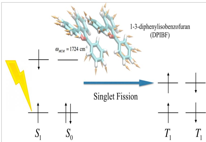
**Figure C.2** Diagram depicting singlet fission. This emerging technology may help improve solar cell efficiency by turning two singlet molecules into two triplet molecules upon the absorption of an incident photon.
