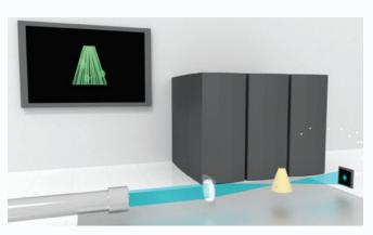
This illustration shows a coherent x-ray beam focused on a large-scale specimen while recording far-field diffraction patterns as the specimen is scanned and rotated. In the background is a computing system using automatic differentiation approaches to reconstruct a 3D image. *Image: Ming Du, Argonne National Laboratory*
