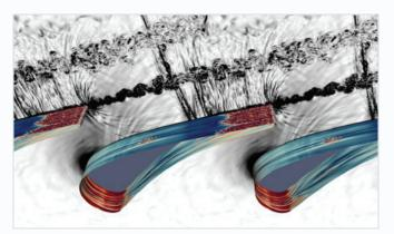
Flow in the transonic turbine inlet guide vane LS89 at Re=1.2 million, computed using 4th-order-accurate DG. The acoustic waves and shock system are visualized via numerical Schlieren, whereas the instantaneous wall heat flux is shown on the suction side. *Image: J. S. Cagnone, M. Rasquin, and K. Hillewaert, Cenaero.*
