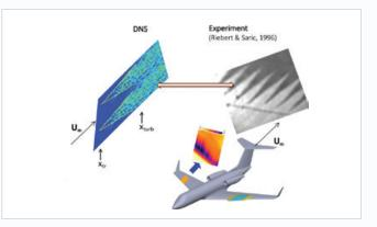
DNS captures swept-wing boundary layer transition over a transonic aircraft with laminar flow technology. Near-wall flow visualizations confirm the sawtooth nature of transition front as a generic feature of transition due to stationary crossflow vortices regardless of the type of secondary instability. *Image: NASA*
