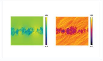
These images show the density fields at a low convective Mach number (left) and a higher convective Mach number (right). At high convective Mach number significant acoustic emission, including eddy shocklets, result from the turbulent mixing. *Image: Sanjiva Lele, Stanford University*
