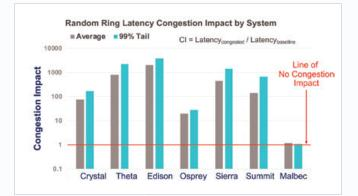
Mean and 99th percentile congestion impact (defined as the latency under congested conditions divided by the latency under isolated network conditions) across a range of systems and architectures for latency. *Image: Sudheer Chunduri, Argonne National Laboratory*
