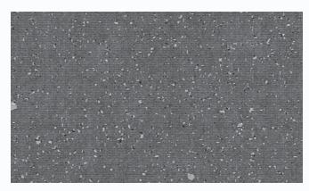
Snapshot from a simulation of helium atoms beneath a tungsten surface to 100 eV helium plasma for 840 ns (fluence of 8.4 x 10<sup>18</sup> m<sup>-2</sup>). *Image: K. D. Hammond, University of Missouri, et al., Nuclear Fusion (2019) vol. 59, no. 6.*
