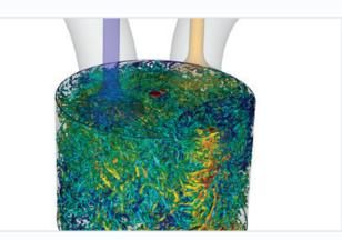
Snapshot of turbulent eddies in the compression stroke during the third engine cycle (1700.5 CAD). Eddies colored by velocity magnitude in the TCC-III internal combustion engine designed by GM. *Image: Argonne National Laboratory*
