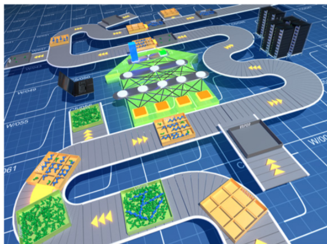
Figure 8.1 Big data from high-throughput simulations and a deep neural network are utilized to find optimal conditions for contracting a solution phase (green box) with a zeolite (orange box) to yield pure liquid solvent and a zeolite with enriched product, followed by partial desorption of the solvent into a vapor phase, leading to essentially pure product that can subsequently be desorbed.
