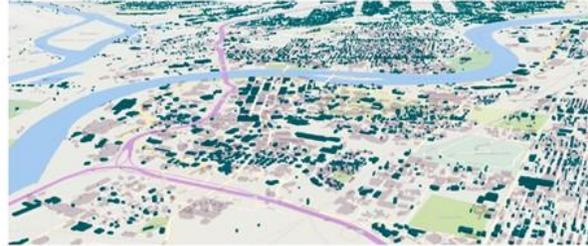
A digital twin of Chattanooga, Tennessee processed with the AutoBEM software. All 178,337 buildings and simulation results can be searched, selected, and visualized using flexible regular expressions at [bit.ly/virtual\\_epb](http://bit.ly/virtual_epb) (Image courtesy of Joshua New).
