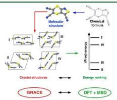
Crystal structure prediction workflow based on the GRACE software for sampling crystal structures and the first principlesbased DFT+MBD framework. (Alexandre Tkatchenko, University of Luxembourg).
