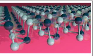
Figure 8.2 Optimized geometry of GeSe monolayer using the newly developed structural optimization algorithm within Quantum Monte Carlo (colored structure) compared to the initial Density Functional Theory-optimized structure (clear structure).
