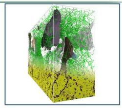
A data reduction workflow in which a detailed all-atom representation of compressed crystal (bottom) gradually morphs into a more economical representation (top) in terms of its lattice defects - dislocation lines and interfaces of twin particles. (Image courtesy of Alexander Stukowski).
