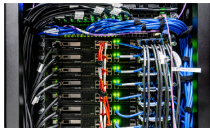
Figure 6: Graphcore Bow : Pod-64 configuration with 64 accelerators
