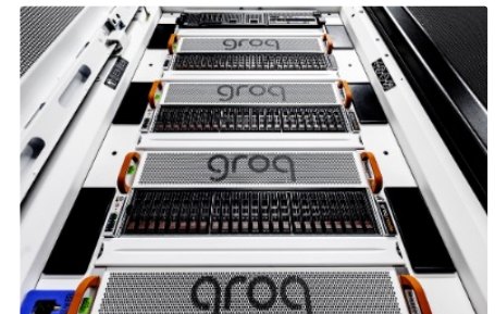
Figure 8: GroqRack : 9 nodes, 8 GroqChip v1.5 Tensor streaming processors accelerators per node
