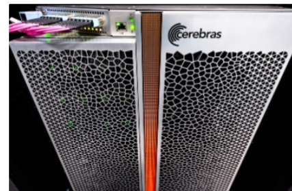
Figure 7: Cerebras : 2x CS-2 WSE with Memory-X and Swarm-X technologies
