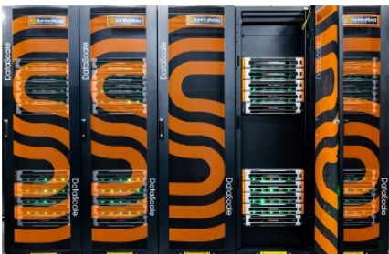
Figure 5: SambaNova SN-30 2nd Gen, 8 nodes with 64 AI Accelerators
