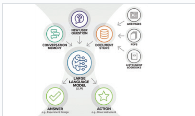
Overview of CALMS: CALMS uses a large language model in conjunction with conversational memory, document stores, and experimental tools to answer user queries or take action to drive an instrument. Image: Prince et al. npj Computational Materials 10, 251 (2024).
